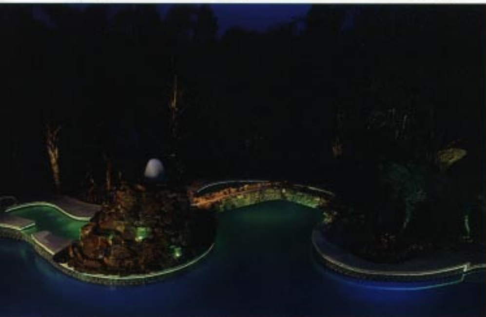
(left) Illumination is provided by three light sources with color changing ability. The sources are remotely switched from the house. (right) The primary cost of a fiber optic system is in the cable. In this project, extremely long cable runs were required, using nearly 300 ft of cable.
