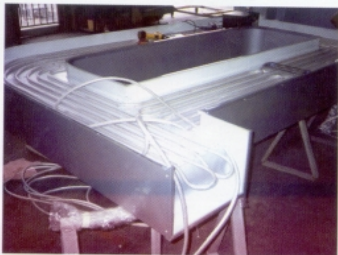
Fig. 2: SuperVision's Sideglow™ FO cables are looped to form six rows in each of the 10-ft. letters.
